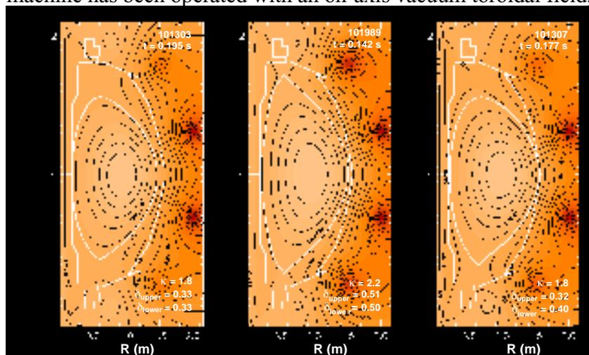
Fig. 1. EFIT reconstructions of poloidal flux contours for limited, double-null, and lower single-null diverted equilibria.
