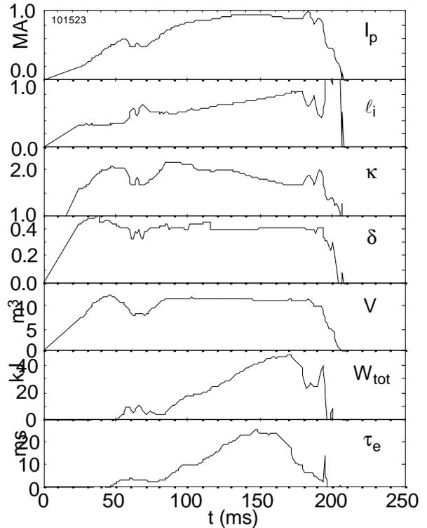
Fig. 2: Time evolution of EFIT reconstructed plasma parameters for a 1 MA ohmic discharge. The interval between reconstructions is 1 ms.
