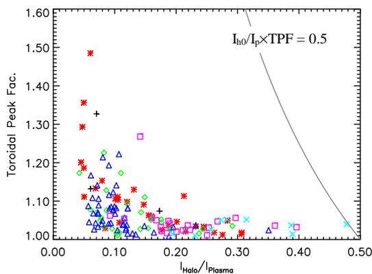
Figure 3: Toroidal Peaking Factor (TPF) for halo currents in P2 supports, calculated at time of maximum halo current. Line indicates typical design constraint for ITER-FEAT [3]
