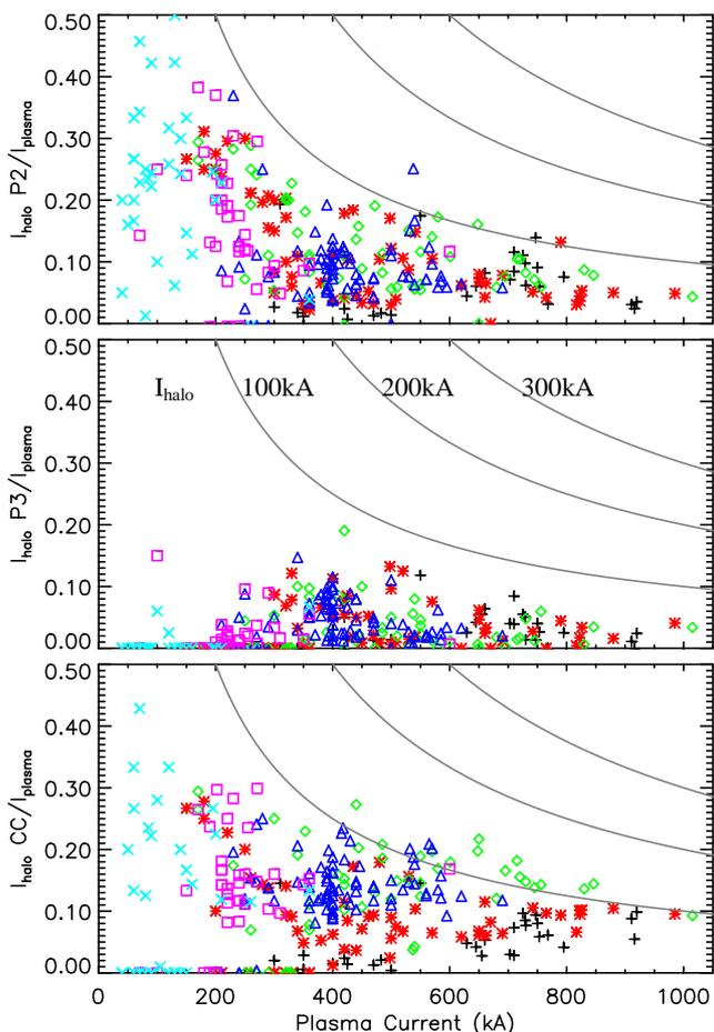
Figure 4: Summary of halo current measurements in MAST. Lines indicate curves of constant halo current. Symbols indicate where in the solenoid cycle the VDE occurred. Start-up, rampdown, flattop and decay phase (+, \*,  $\Delta$ ,  $\times$ ) and also those triggered by rapid changes in loop volts ( $\diamond$ ,  $\square$ ).
