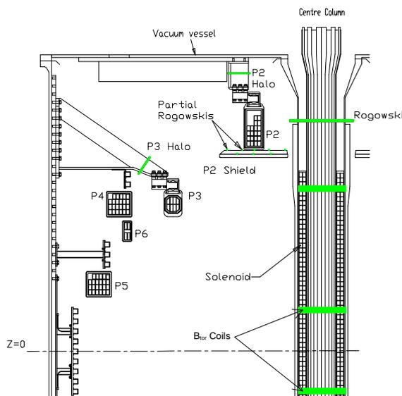
Figure 1: Schematic of MAST vessel showing position of halo current detectors
