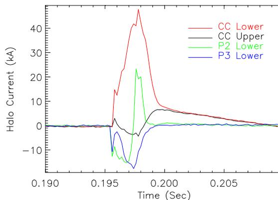
Figure 2: Total halo currents measured in P2/P3 Supports and centre column for a downwards VDE,  $I_p \sim 390kA$  (shot 2223)
