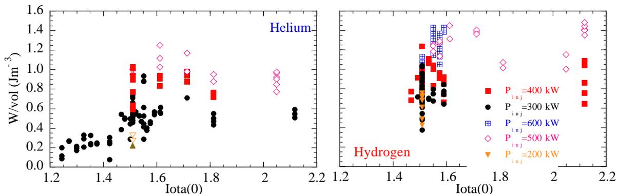
**Figure 2:** Evolution of diamagnetic energy content normalised to the calculated configuration volume as a function of rotational transform for helium and hydrogen plasmas and several values of heating power.
