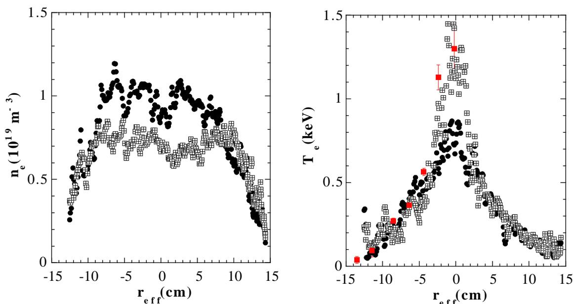
**Figure 3:** Thomson scattering profiles of helium plasmas with injected power of 300 kW, rotational transform  $iota(0)=1.51$  and different electron density. ECE temperature profile is displayed for the low density case in which the ITB appears.
