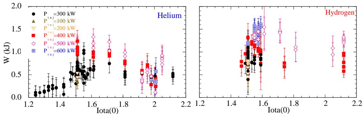
**Figure 1:** Evolution of diamagnetic energy content as a function of rotational transform for helium and hydrogen plasmas and several values of heating power.
