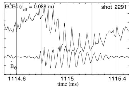
**Figure 3.** Temporal evolution of one of the ECE channels (corresponding to  $r_{\text{eff}} = 0.088\text{m}$ ) and of the Mirnov coil signals during an ELM-like event, in discharge #2291.
