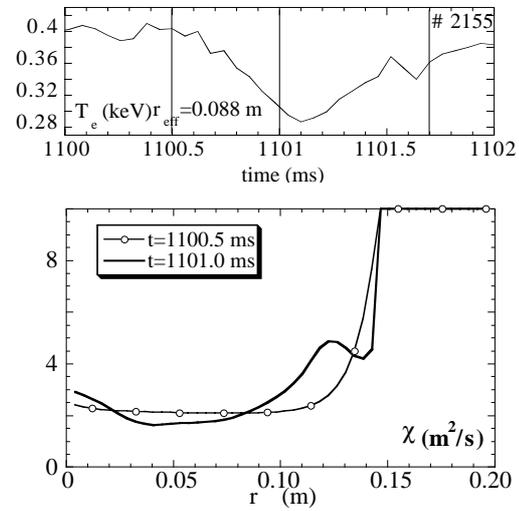
**Figure 2.** Electron conductivity profile for the evolution of the single ELM-like event.
