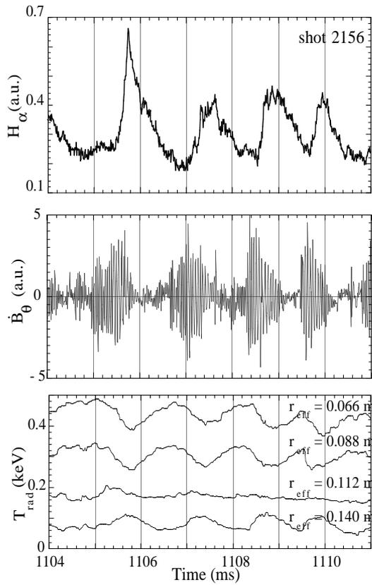
**Figure 1.** Time traces of: (a)  $H_{\alpha}$  signal, (b) Mirnov coil signal and (c) ECE signals at four radial positions showing ELM-like activity in TJ-II shot #2156.
