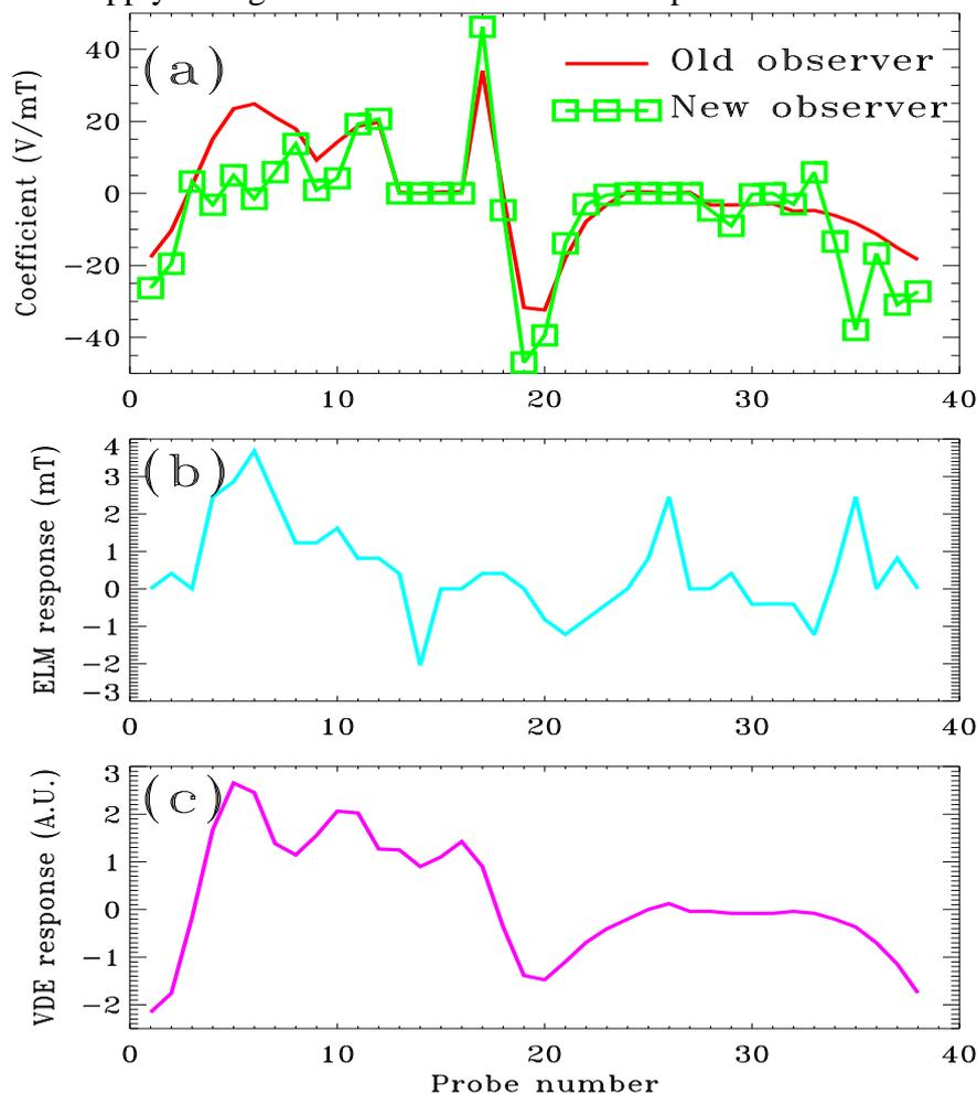
Fig.3.: (a) Old and new observer coefficients vs. probe number, (b) ELM response (Shot 18329 at 0.76s), including effect of internal active coils (peaks at #14 and #26), (c) Response of a VDE (Shot 15971 at 0.605 s). The VDE was intentionally produced by a preprogrammed feedback cut.
