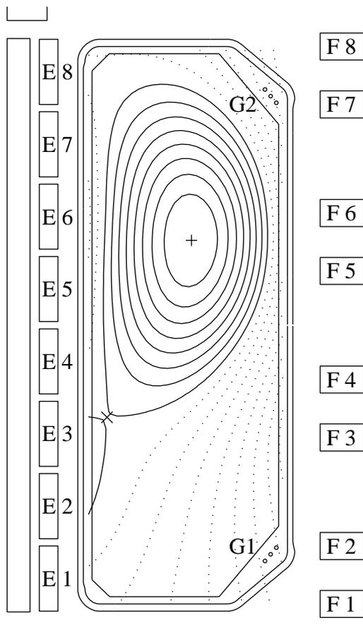
Fig.1. ELMy H-mode plasma in TCV: Shot # 18416 at 0.57 s,  $I_p=513\text{kA}$ ,  $B_{tor}=1.45\text{T}$ ,  $\kappa=2.03$ ,  $\delta=0.45$ , ELM frequency=170 Hz. Feedback for vertical position control is applied to coils F3, F4, F7, F8, G1 and G2.
