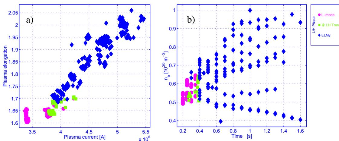
**Figure 3:** a) Accessible plasma current and elongation for the ELMy H-mode. b) Accessible plasma density for the ELMy H-mode. In both cases these parameters may only be obtained after passage through the ELMy “gateway”.
