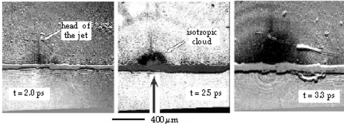
Fig. 3: Shadowgraphy images. The arrow shows the direction of the laser pulse.
