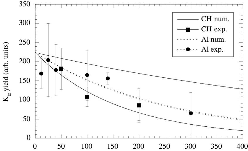
Fig. 2: Results at LULI in the high intensity case ( $T_{hot} = 400$  keV): experimental and numerical  $K_\alpha$  yield vs. target thickness in  $\mu\text{m}$ , and interpolation ( $\exp(-R/R_0)$ )
