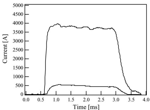
Fig. 3 Current signals (high: primary current, low: ionization chamber current)
