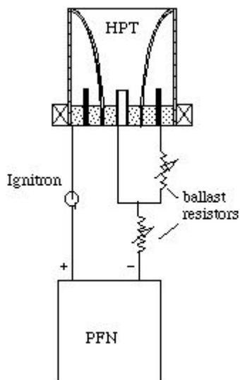
Fig.2 Main electric circuit arrangement
