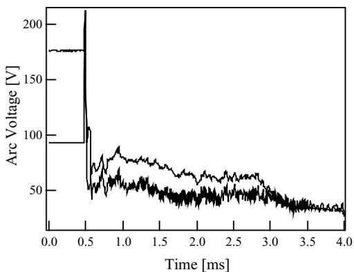
Fig. 4 Voltage signals (high: primary voltage; low: ionization chamber voltage)
