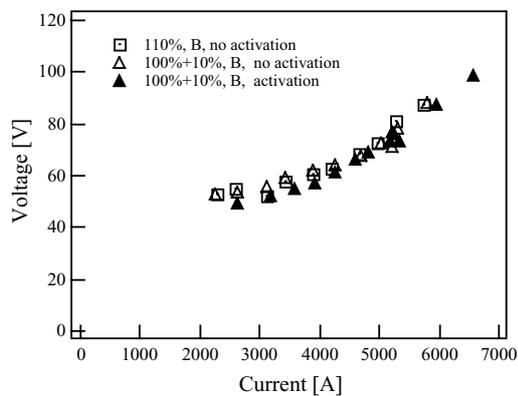
Fig. 5 Electrical Characteristics (660 mg/s, argon)
