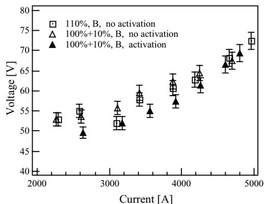
Fig. 6 Electrical Characteristics (660 mg/s, argon, zoom)
