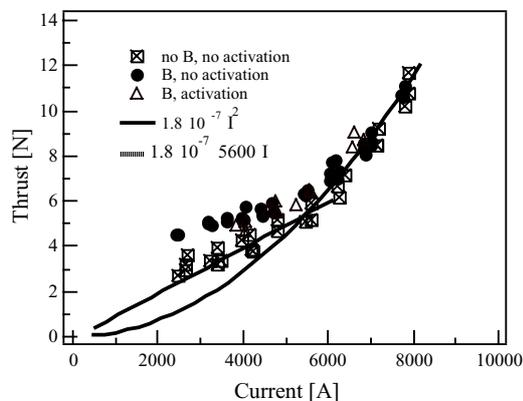
Fig. 7 Thrust vs Current (660 mg/s, argon)
