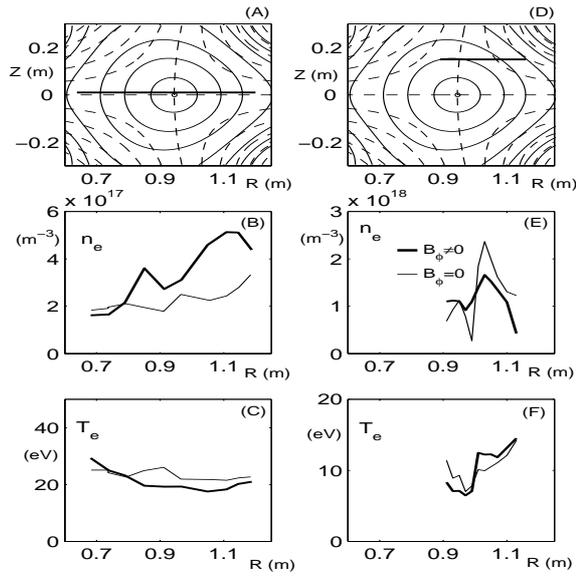
**Fig.2** Plasma profile measurements with Langmuir probes. A, D: probe location. B, C, E, F: density and temperature measurements, with and without a toroidal field.
