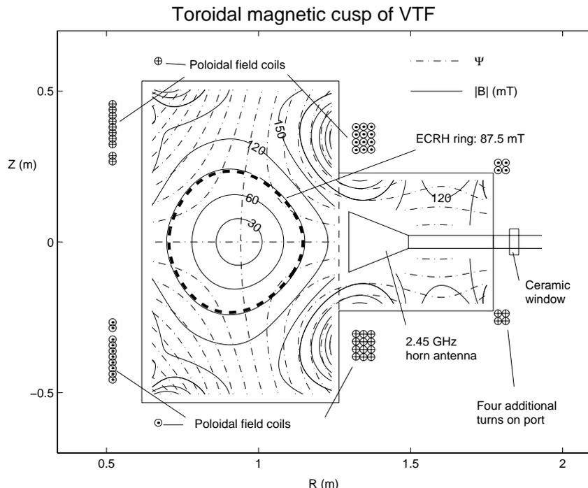
**Fig.1** VTF cross section. The solid contours represent the poloidal magnetic field strength. The dashed contours correspond to constant levels of poloidal magnetic flux.
