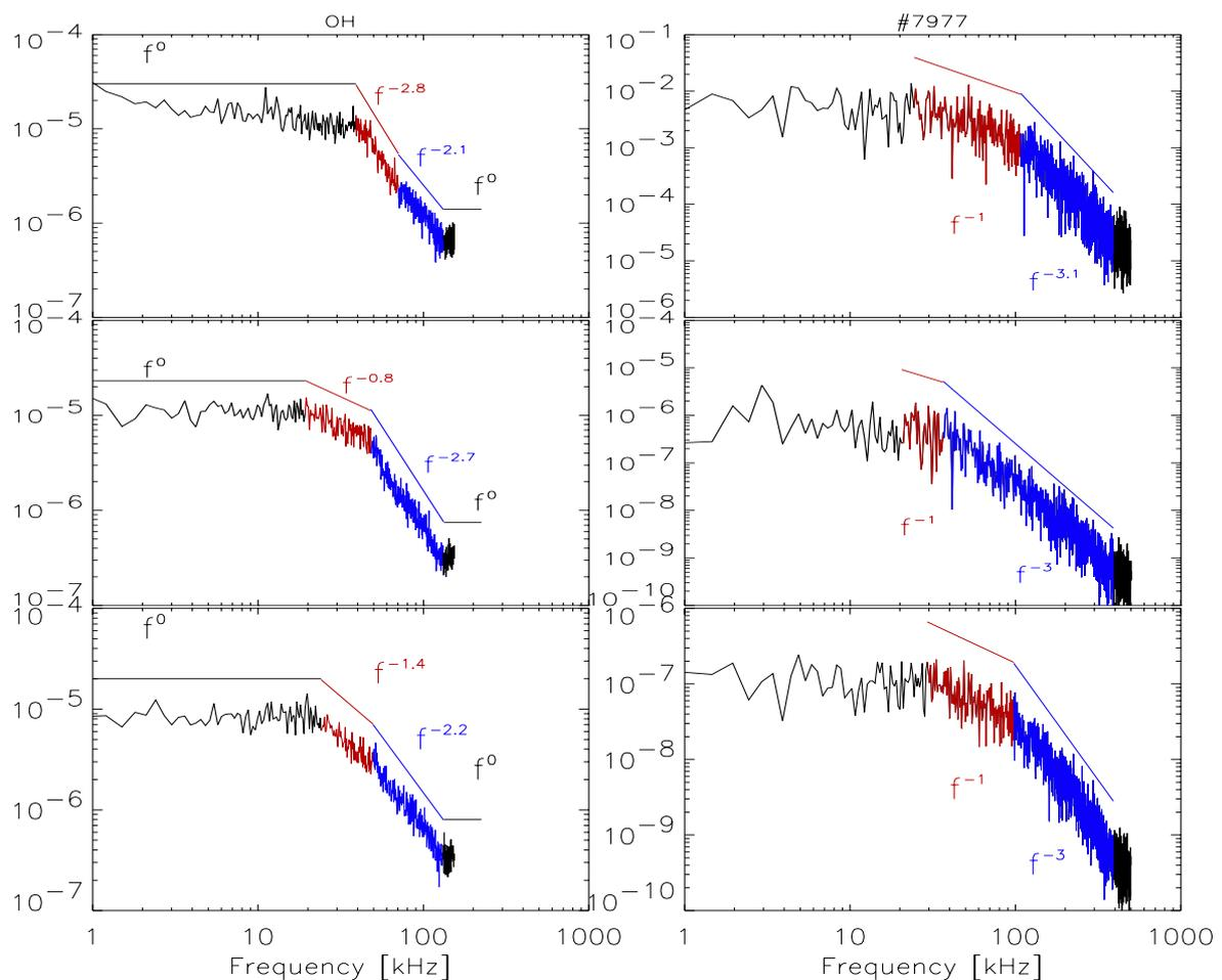
Figure 2. Left column: Power spectra of  $U_{fl}$  fluctuations: top - 5 mm inside VSL, middle - at VSL and bottom - 5 mm outside VSL, measured by radial array of LPs. Right column: Power spectra (from top to bottom) of  $E_\theta$ ,  $I_{sat}$  and  $\Gamma$  all at VSL, measured by poloidal array of LPs.
